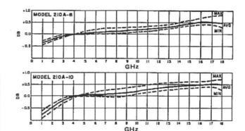
CALIBRATION FREQUENCIES: Certificate supplied giving insertion loss in 50-ohm system at 1.0, 4.0, 10.0 and 18.0 GHz up to 10 dB, and at 2.0, 4.0, 10.0, and 18.0 GHz for 20 dB. SWR is guaranteed to be within specified limits.
