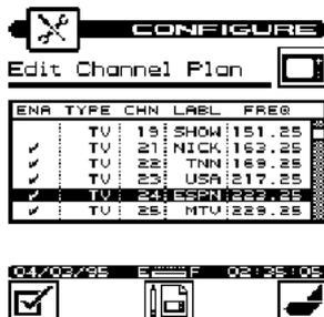
You must enable a channel in order to perform measurements on it. A check mark appears in the left-hand column when the channel is enabled. When you built the plan, microStealth automatically enabled all the channels it found to be active on your system. You may want to verify that all your channels have been correctly enabled. Use the  soft key to enable/disable the channel highlighted in the list.
