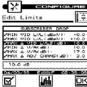
You can selectively enable or disable each individual limit. When a limit is disabled, your microStealth excludes it when checking limits. If the highlighted limit is disabled, you can enable it by pressing the soft key. A check mark appears in the left-hand column to indicate when a limit is enabled. If the limit is already enabled, pressing the soft key disables it.
