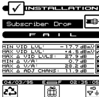
To quickly determine the status of the overall limit check, look at the PASS/FAIL indicator located in the upper portion of the screen. This indicates FAIL if any channel is not within the required limits. For each limit, the worst case actual value is displayed along with a pass/fail status.
