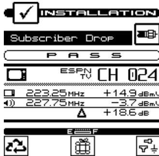
This screen displays video and audio carrier level measurements along with the DVA for the selected channel. Use the up or down arrows to select the previous or next channel in the list.
