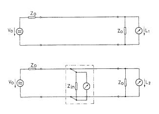
The bridging loss is defined as follows: Bridging loss  $a_B = L_2 - L_1$
