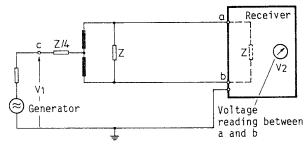
Receiver signal balance ratio is defined as:
