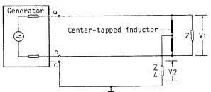
Generator signal balance ratio is defined as:
