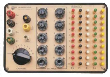
features locking potentiometers, but without turns-counting dials. (SB-10 front panel is shown).
