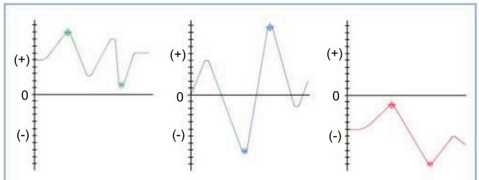
The Model 3650 simultaneously displays both the maximum (most positive excursion) and minimum (most negative excursion) values of a transient waveform, as illustrated in the above diagram.
