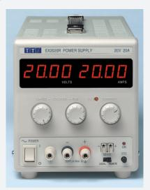
Switchable remote sense is provided to remove the effects of connection lead resistance at high current.
