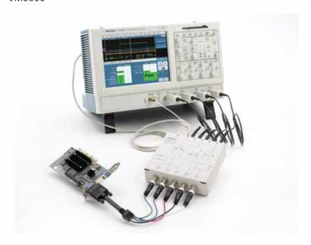
The VM5000 automates video testing of consumer HDTV and PC graphics devices such as digital set-top boxes, multi-media PCs, graphics cards and video semiconductors. It addresses the needs of engineers developing and deploying the next generation of video devices for the digitally connected home. Unrivaled performance in terms of speed, accuracy and reliability has made the VM5000 the choice of industry leaders for design validation, quality control and ATE applications.
