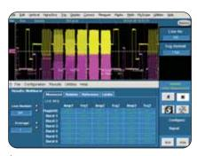
Multiburst Measurement Results Display (Option SD and HD).
