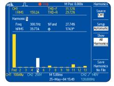
Conduct harmonic distortion measurements with TPS2PWR1 software.
