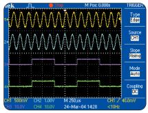
Four IsolatedChannel<sup>™</sup> inputs and isolated external trigger input for quick, accurate, affordable floating and differential measurements.
