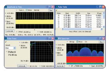
Pulse measurements, available in the Advanced Signal Analysis package (Opt. 20): A pulse train (upper left) is seen with measurements of peak power, pulse width, rise time and pulse-to-pulse phase (upper right). A detailed view of the pulse rise time is seen in the lower left and a DPX display monitors the spectrum on the lower right.
