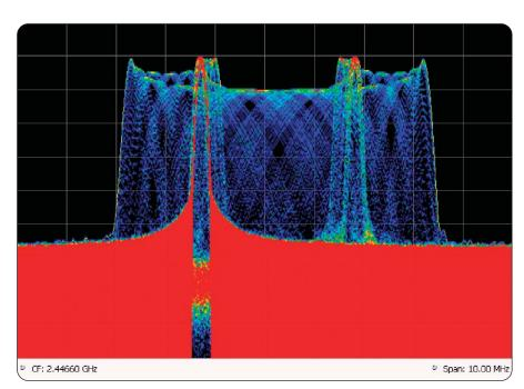
Revolutionary DPX spectrum display reveals transient signal behavior that helps you discover instability, glitches and interference. Here, an infrequently occurring transient is seen in detail. The frequency of occurrence is color-graded, indicating the infrequent transient event in blue and the noise background in red.
