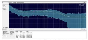
Phase noise and jitter measurements (Opt. 11) on the RSA5000 Series may reduce the cost of your measurements by reducing the need for a dedicated phase noise tester. Outstanding phase noise across the operating range provides margin for many applications. Here, phase noise on a 13 MHz carrier is measured at -119 dBc/Hz at 10 kHz offset. The instrument phase noise of < -134 dBc/Hz at this frequency provides ample measurement margin for the task.
