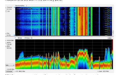
DPX Spectrograms provide gap-free spectral monitoring for up to days at a time. 60,000 traces can be recorded and reviewed, with resolution per line adjustable from 125  $\mu s$  to 6400 s.
