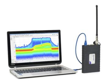
The RSA306 uses your PC and Tektronix SignalVu-PC<sup>™</sup> RF Signal Analysis Software to provide real time spectrum analysis, streaming capture and deep signal analysis capabilities for signals from 9 kHz to 6.2 GHz, all in a low-cost, highly portable package that is ideal for field, factory, or academic use.
