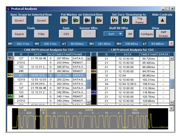
CAN and LIN Timing and Protocol Decode
