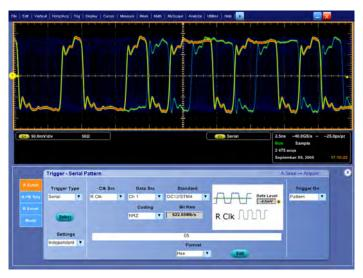
Serial pattern triggering to debug pattern-dependent issues.
