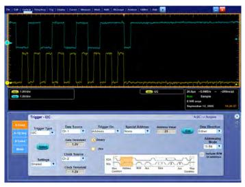
Easily trigger on a specific I2C address.
