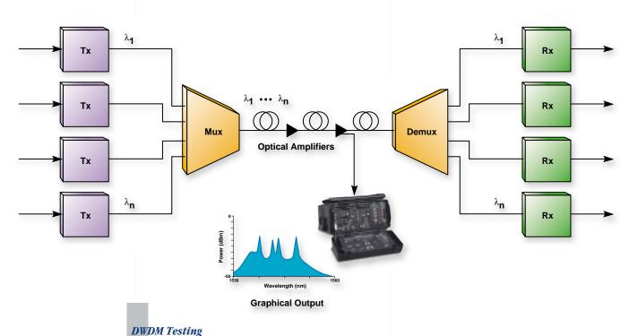
Use a printer or laptop computer to tabulate and graph all the channels in the DWDM system. View the graphical output to determine gain tilt and power flatness of the optical amplifiers to ensure equal distribution of power in all channels.
