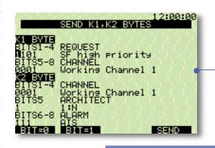
Advanced users can control/read Sonet overhead bytes. The english decodes make overhead simple.
