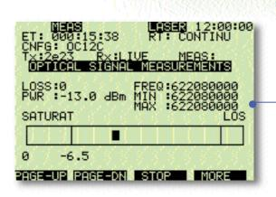
Field operators can quickly verify signal level with an easy to read power measurement.
