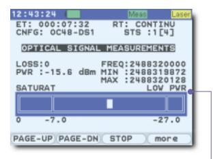
Field operators can quickly verify signal level with an easy to read power measurement.
