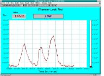
*Leak detection mode* monitors a particular mass number (not just helium) over time, and combines many features of the previous modes. A vertical bar graph provides a visual reference for viewing changes in intensity from a distance. A programmable audible tone, large numeric read-out, and visual alarm are also provided.
