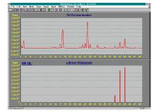
*Library mode* contains a comprehensive list of gases that can be used to compare against the current spectrum. A search mode allows you to select up to 12 masses and identify and display (numerically and graphically) the intensity of all gases that contain these masses.
