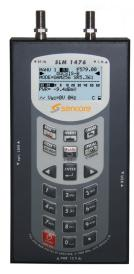
The SLM 1476CM provides everything installers and operators are looking for in a signal level meter. Capable of analog and digital measurements, including Pre/Post BER, MER, Spectral Display, DOCSIS 2.0 Network Testing, and Leakage and Ingress Testing capabilities all at an affordable price. Designed to easily test multiple DOCSIS channels. The SLM 1476 provides a pass/fail test which can be logged.
