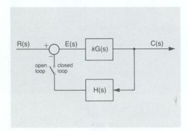
The 1250 Series Frequency Response Analysers are designed to provide the control systems design engineer with an optimised measurement system to analyse the performance parameters of servo systems, hydraulic actuators, electromechanical components, etc. Its unique method of single sine correlation ensures that the fundamental components of the system response are analysed, without corruption by associated harmonic and noise signals.
