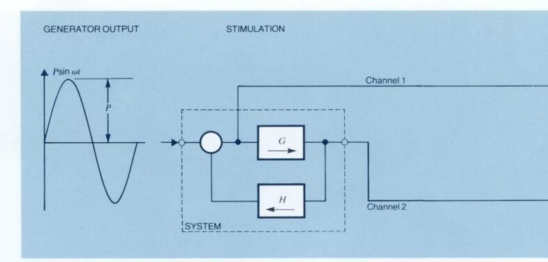
The device under test is stimulated by a sinewave and the response analysed at one, two or more points in the system. These responses are then correlated with the stimulus to determine the amplitude and phase relative to the generator. The ratio of the two measured signals can then be calculated to provide the system transfer function.
