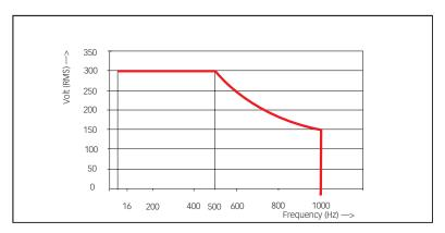
Voltage Vs frequency de-rating curve
