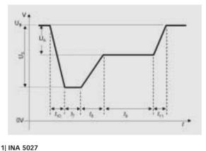
Simple ISO-type pulse 4 and 2b are programmable in the most cost-effective way.
