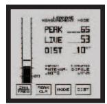
Find leakage problems quickly using the search mode. Change to the measurement mode to accurately measure the leakage value based on your distance to the leakage source.
