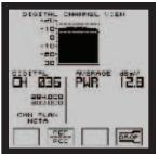
Quickly tune and display the average power of a single digital channel. The spectrum analyzer display shows how the power is distributed over the channel's bandwidth.
