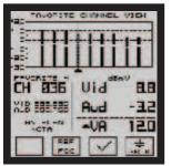
View only 'Favorite' channels for a quick snap-shot of the system. Press the 'check' key for an on-screen pass/fail summary.
