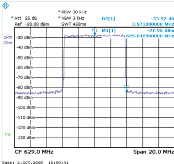
Frequency spectrum with transducer function.
