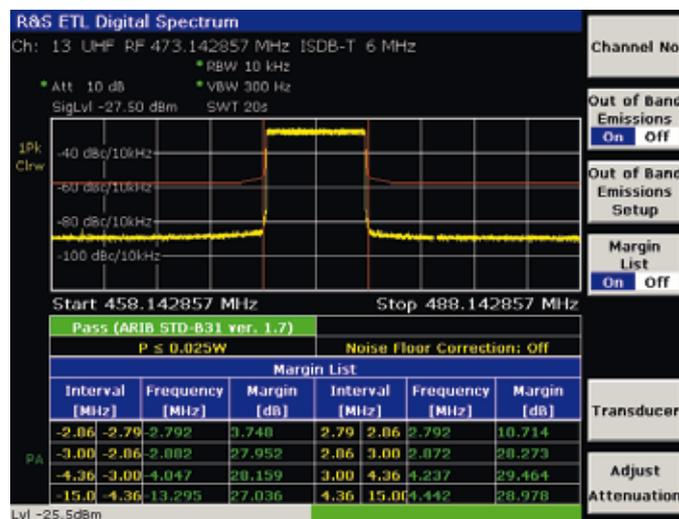
Shoulder attenuation measurement in line with ETSI TR 101290.
