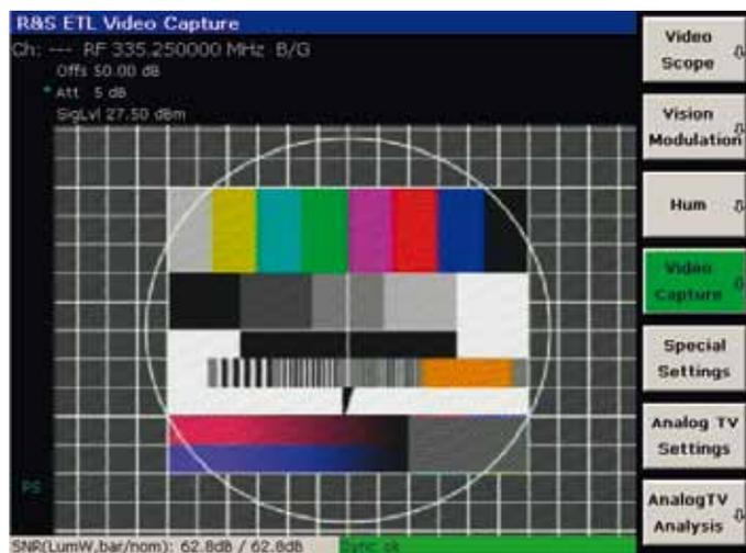
Video test line with measurement parameters.
