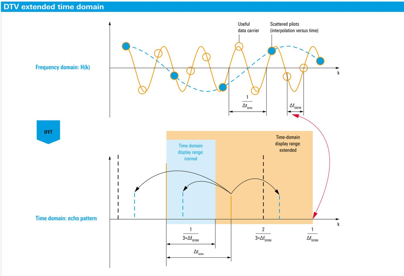
A special feature of the R&S®ETL is the positioning of the FFT window. To help ensure stable synchronization to the transmitter signal, especially for field measurements, the R&S®ETL tries to place all impulses above an echo detection threshold so that they are equidistant within the guard interval. For some applications, the echo detection threshold is dependent on the system optimization method selected by the user.
