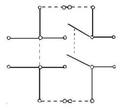
20 independent relays. 1 channel is shown, with provision for addition of series and shunt elements.
