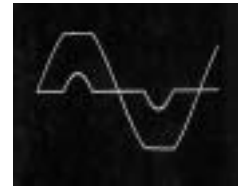
Oscilloscope of voltage and current waveform at load due to distribution losses. THD=6.6%
