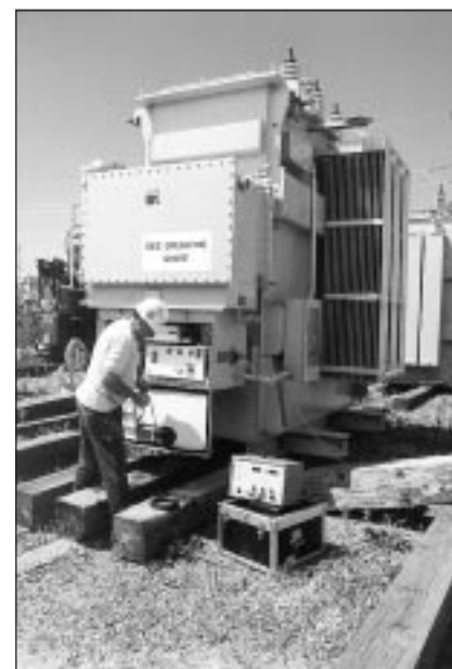
Power utilities can reduce expensive downtime by early detection of tap-changer problems using the Multi-Amp Transformer Ohmmeter.
