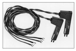
Cat. No. 242011-7 Duplex Helical Current and Potential Hand Spikes. These optional helical hand spikes have pyramid-pointed prods backed by stout springs and helical guides that rotate the prods when pressure is applied to the handles. This feature ensures good contact and allows operation at precise angles. Maximum allowable test current is 20 A.
