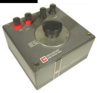
The Leeds & Northrup 4385 Shunt Box is a precision bench top instrument for current measurement up to 15 amps. Bifilar and folded construction on the elements provides good AC/DC agreement up to 1000 Hz.
