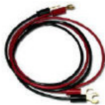
CAB024: The CAB024 is a low thermal EMF spade lug patch cord set for low voltage measurements. These low thermal cables minimize thermal errors so accurate low voltage measurements can be made. Each set includes 2 test leads (one black and one red).
