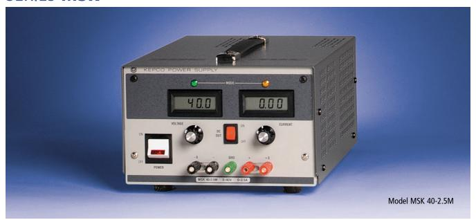
Kepco's MSK linear power supplies provide a selection of five models, offering 100 Watts of stable benchtop power. They use a high gain linear (series pass) stabilizer circuit for low noise output, good stability, and accurate resettability.
