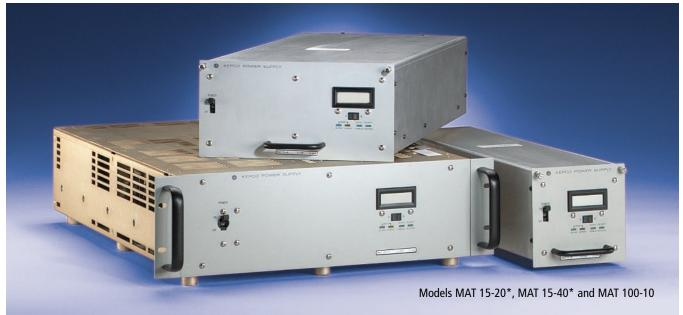
Kepco MAT power supplies are oriented to systems applications. Their principal control means is a 2-wire, long range, serial bus, Kepco's single address, multiple instrument bus. As many as 27 power supplies, including models in the Kepco MST and BOP series may be "daisychained" on this bus and interfaced either to IEEE 488.2, a PC bus, or to a VXI host.
