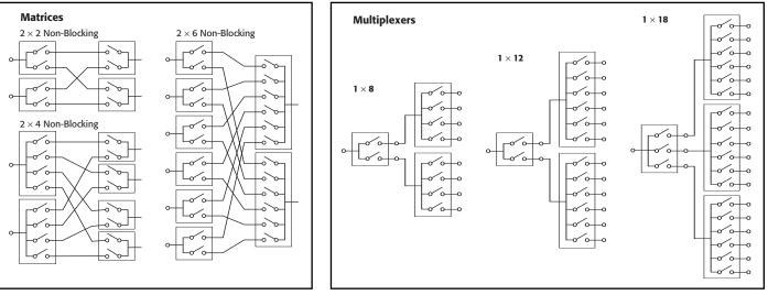
MAXIMUM CONFIGURATION: (8) - Unterminated SPDT relays. (4) - Unterminated multi-pole relays (SP4T, SP6T)
