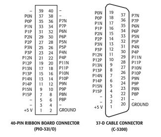
For pin assignments of channels 16-31, add sixteen to the channel numbers shown, (i.e. PON becomes P16N, etc.)
