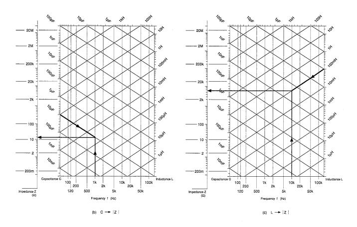
Figure A-1. Conversion Diagram from L or C to |Z|
