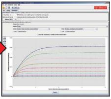
Performing nested sweeps to characterize a transistor with TSP Express is quick and easy. Data can be exported to a .csv file for use with spreadsheet applications such as Excel.
