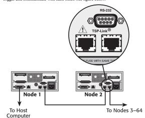
Each SourceMeter instrument has two TSP-Link connectors to facilitate chaining instruments
