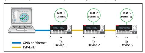
Parallel testing with the Series 2600A
