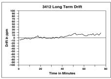
With a typical drift of less than 20 ppm/°C over a 30 min period, the LDX-3412 out-performs typical low-cost power supplies
