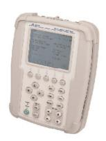
The IFR 4000 is a compact, lightweight and weatherproof unit designed for testing ILS, VOR, Marker Beacon and VHF/UHF Communications avionics systems.
