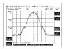
The tracking generator facility (with offset tracking) is provided for RF module characterization. With a useable frequency range of 100 kHz to 1 GHz and 1.3 GHz to 2.2 GHz, the spectrum analyzer supports IQ modulator alignment and the testing of internal local oscillators and IF systems. IQ alignment tests are recommended on most popular GSM terminals.
