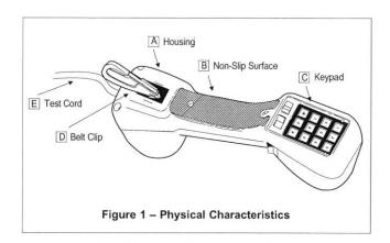
(e) The test sets are equipped with several different cord configurations (E). The line cords may be replaced in the field (see sections 4 and 6.02).
