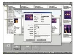
Assign a unique name, preset emissivity and RTC values, assign alarm limits and add meaningful comments to each measurement location.
