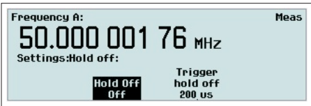
Fig. 2-13 The trigger hold-off submenu.
