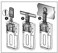
Hang your Fluke 180 Series meter by a magnet or strap hanger with the optional ToolPak<sup>m</sup> accessory.
