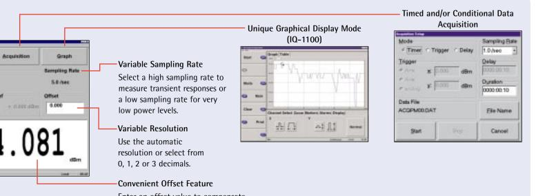
Enter an offset value to compensate for known power loss or gain.
