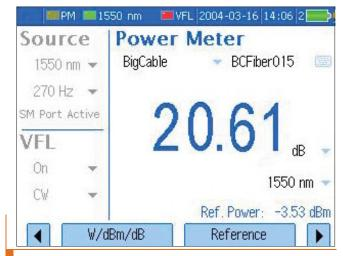
The FOT-930 lets you use a high-power source, a high-power power meter, as well as a talk set and visual fault locator combination, all at once.
