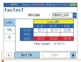
In 10 seconds, the MaxTester's FasTest function provides insertion loss and ORL values for up to three wavelengths—including either 1490 or 1625 nm—on a single port.
