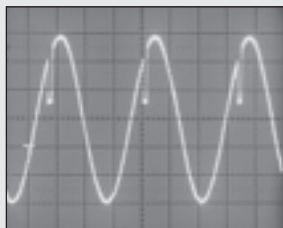
Sine wave with a dropout from 45° - 60°
