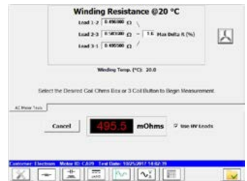
\mu\Omega measurement of 3-phase motor
