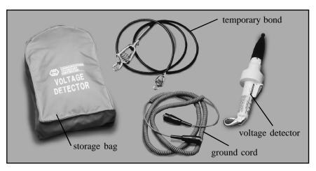
Figure 2: Voltage Detector and Accessories
