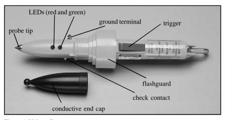
Figure 1: Voltage Detector
