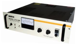
Spellman's Bertan brand of 210 Series of 125 to 225W high voltage power supplies provide regulated high voltage outputs from 1 to 50kV. The low noise, linear topology employed results in extremely low output ripple specifications. Units are inherently reversible by design, providing either positive or negative output polarity. The 210 is fully arc and short circuit protected. Excellent regulation specifications are featured along with outstanding stability performance.
