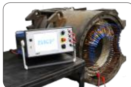
Testing individual coils within the stator.
