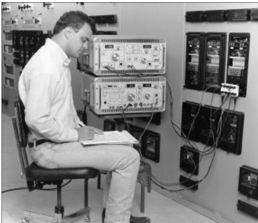
Model SR-90, with Units 1 and 2 stacked, tests a current differential relay in a panel.
