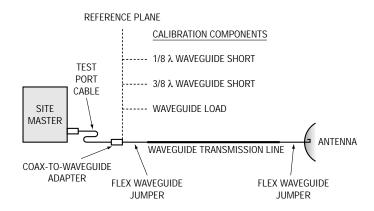
Vector Correction Avoids Bulky Waveguide Coupler
